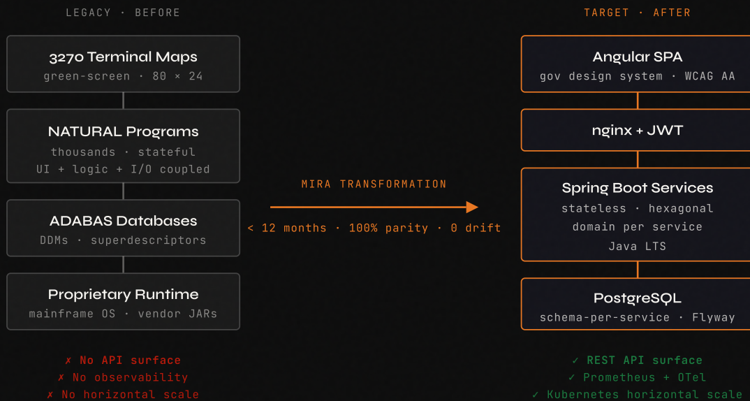
FIGURE 3 · LEGACY MAINFRAME STACK VS. CLOUD-NATIVE TARGET ARCHITECTURE
