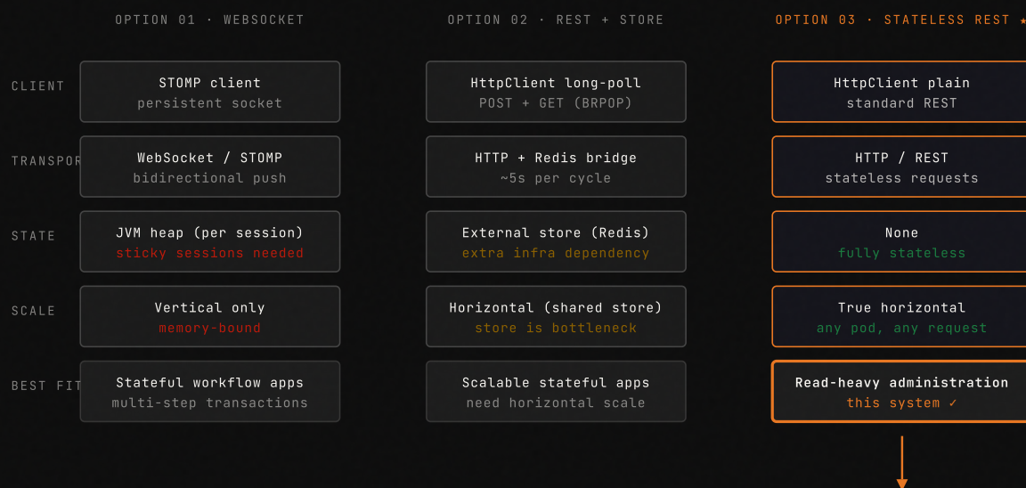
FIGURE 2 · THREE OPTIONS FOR THE STATEFUL → STATELESS TRANSITION. CHOSEN PATH HIGHLIGHTED.
